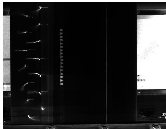
Figure: 6 Triangular VG (h=3mm, z=9\text{mm} ) 0^\circ deflected flap, \alpha = 15^\circ
